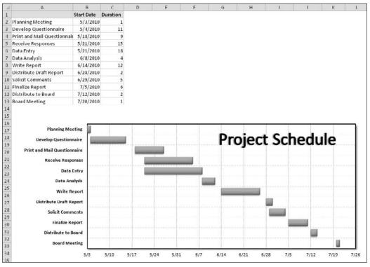
Figure 137-1: You can create a simple Gantt chart from a stacked bar chart.
