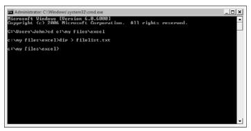
Figure 181-1: Using the Windows command prompt to generate a list of files.
