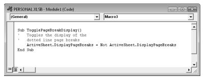
Figure 206-1: A simple, but useful, VBA procedure.
